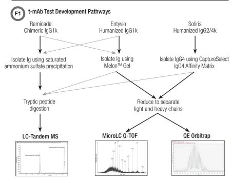
Using three examples of tests implemented in clinical laboratories, different enrichment and detection techniques using mass spectrometry are shown. The gray arrows show the versatility of the techniques that may facilitate future t-mAb test development.
